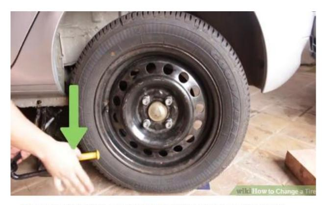
13 Lower the car to the ground fully and remove the jack. Finish tightening the nuts and replace the hubcap.
