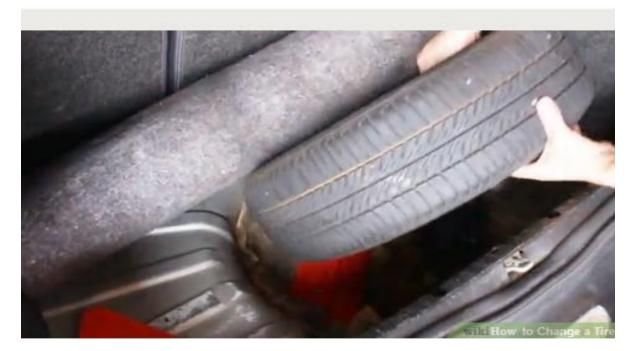
Take out the spare tire and the jack. Place the jack under the frame near the tire that you are going to change. Ensure that the jack is in contact with the metal portion of your car's frame
