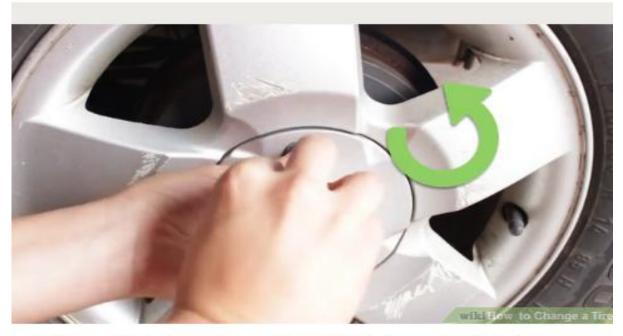
Remove the hubcap and loosen the nuts by turning counterclockwise.
