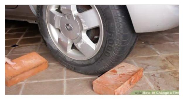
3 Place a heavy object (e.g., rock, concrete, spare wheel, etc.) in front of the front and back tires.
