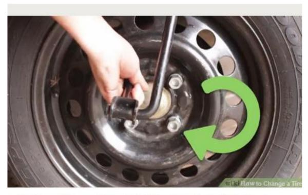
12 Lower the car without applying full weight on the tire. Tighten the nuts as much as possible.
