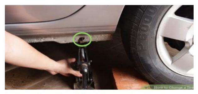
Raise the jack until it is supporting (but not lifting) the car. The jack should be firmly in place against the underside of the vehicle. Check to make sure that the jack is perpendicular to the ground.
