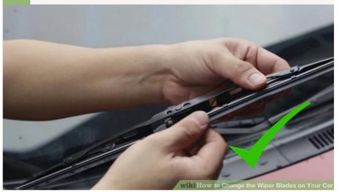
1 Examine the wipers for cracks. Old windshield wipers become hard and cracked over time, especially in hot, dry climates. If your wiper seems to have lost it's rubbery spring, it's probably time to replace it.
