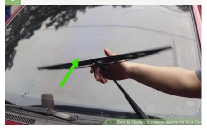
Raise the metal wiper arm away from the windshield. It should be able to hold steady in a position perpendicular to the windshield. Be careful with the positioning; the metal wiper arm is spring-loaded, and it could snap back and crack your windshield.
