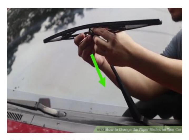
3 Insert the new wiper. Slide the refill wiper into the same end of the arm where you pulled the old wiper out. Gently pivot the new wiper until the hook snaps into place to secure it. Lay the wiper back against the windshield.
