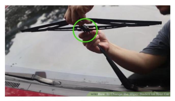
Unhook the old wiper blade. Look at the joint where the rubber wiper blade meets the metal arm. There should be a small plastic stopper holding the blade in place.
