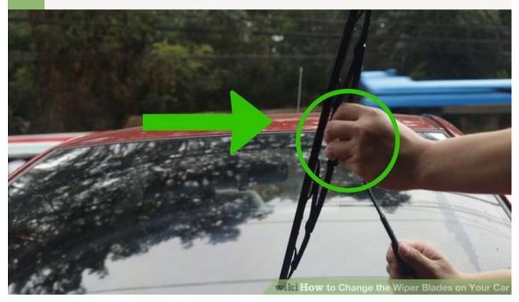
Know what part of the blade to change. Windshield wipers are made with three basic parts: the lower wiper arm that extends from the base of the windshield, the metal or plastic blade attached to the lower arm, and the rubber blade that actually wipes the windshield. When your windshield wiper blades are changed, you're really only changing the rubber blades that get worn down by water and inclement weather.
