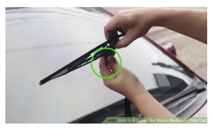
Repeat with the second wiper. The procedure is exactly the same for replacing the second wiper. Just make sure you use the correct size for each side.
