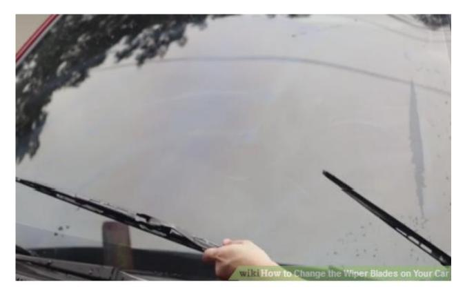
Measure the size blade you need and buy replacement blades. To find out what size replacement blades you need, measure the old rubber blades using a ruler or measuring tape. Write down the exact measurements, then go to an auto parts store and buy rubber blades in those exact sizes.
